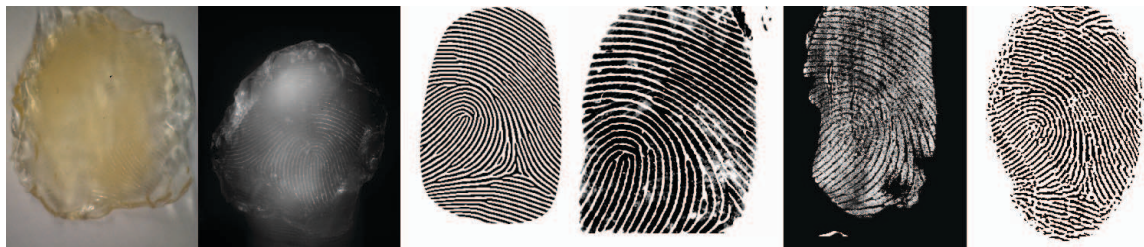
Fig. 17. Latex spoofs images (Dinolite, TBS, original fingerprint, Secugen, BMF Lumidigm).
