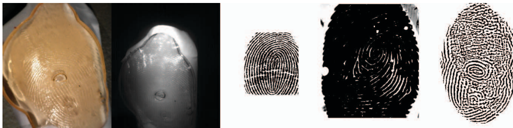
Fig. 15. Gel wax spoofs images (Dinolite, TBS, original fingerprint, Secugen, Lumidigm).
