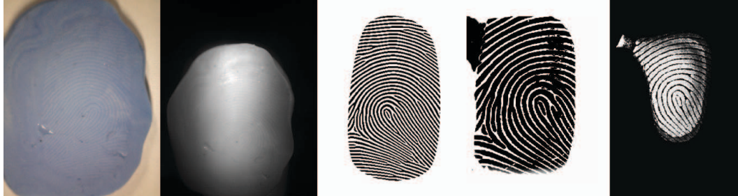
Fig. 18. Siligum spoofs images (Dinolite, TBS, original fingerprint, Secugen, BMF).
