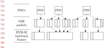
**Figure 6.** The figure shows the encapsulation of network layer PDUs into GSE packets and transmission of GSE packets inside physical layer baseband frames. GSE packets and baseband frames consist of a header (shown as a grey block) and a data field (shown as white space). GSE packet carrying the last fragment also contains CRC-32 (shown as a block with pattern). The figure is based on GSE protocol specification [8, p. 10].
