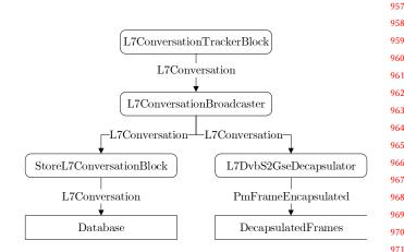
**Figure 9.** Scheme illustrating the connection of *L7DvbS2GseDecapsulatorBlock* to the frame processing pipeline using *BroadcastBlock* placed between *L7ConversationTrackerBlock* and *StoreL7ConversationBlock*. Standard pipeline topology is shown in Figure 4.
