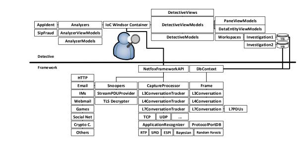
Figure 1. The figure describes the abstraction of OUR TOOL and OUR FRAMEWORK architecture. The upper part of the diagram above the line represents visual parts of the tool. Below the line, components of OUR FRAMEWORK are drawn in a hierarchical view.
