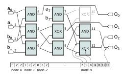
Fig. 1. A two-bit multiplier represented in CGP with parameters:  $n_i = n_o = 4, n_c = n_r = 3, n_a = 2, \Gamma = \{0^{identity}, 1^{not}, 2^{and}, 3^{or}, 4^{xor}, 5^{nand}, 6^{nor}, 7^{xnor}, 8^{cont0}, 9^{const1}\}.$
