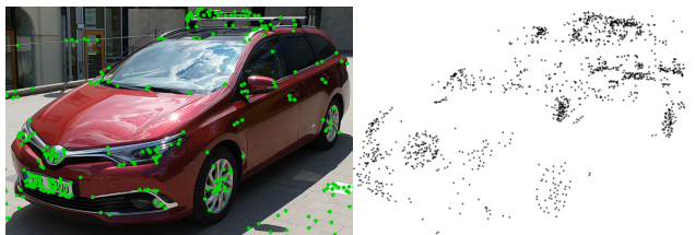
Fig. 11 SfM reconstruction of a particular vehicle model, later used for accurate landmark localization. left : one frame of the source video, with the keypoints marked by green, right : reconstructed point cloud; points are candidate landmarks for the calibration.
