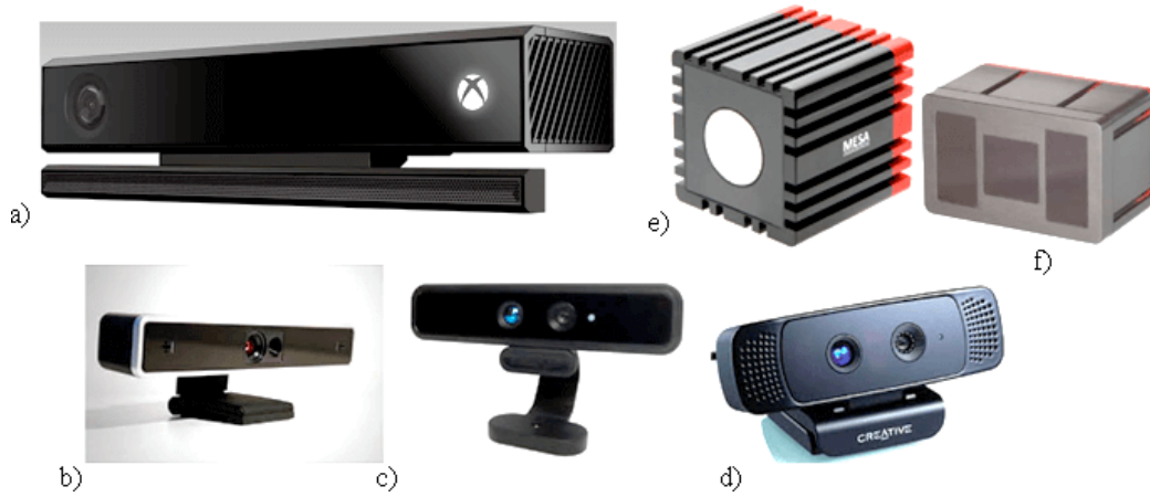
Figure. 5) ToF cameras [26][29]: a) Microsoft Kinect v2; b) SoftKinetic DS311; c) SoftKinetic DS325; d) Creative Sens3D; e) MESA Imaging SR4000; f) MESA Imaging SR4500
