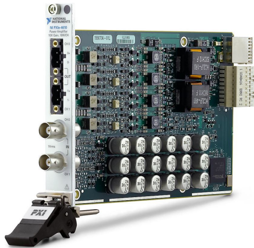
Figure 6.8: The power supply fo Helmholtz coil from the National Instruments company. Taken from [57].
