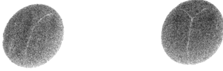
Fig. 3.5: Both the vortex-pair state (left) and the buckling state (right) captured in two D = 2 \mu\text{m} , t = 100 \text{ nm} disks neighboring in the same array. Although the geometry of both disks is identical, their shapes in the images are different because of the high defocus. Note that the magnetic field is pointing in the horizontal direction and that the vortex-pair state is at the stage corresponding to Fig. 3.4(a).
