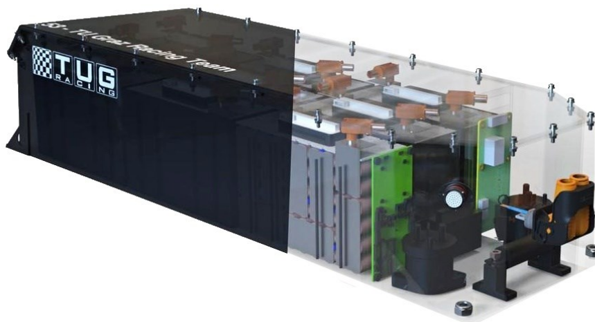
Obr. 7 Formul Student team TUG – hliníkový battery pack [24]
