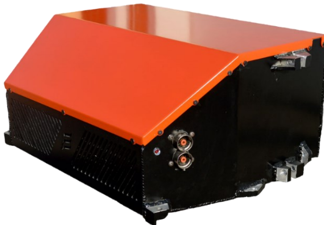
Obr. 6 Formula Student team Illini Electric - oceľový battery pack [23]
