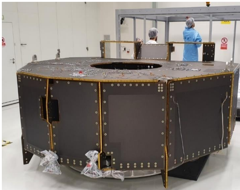
Fig. 7: PLATO SVM test model integration in company's cleanroom in Brno (published with permission of SAB Aerospace)
