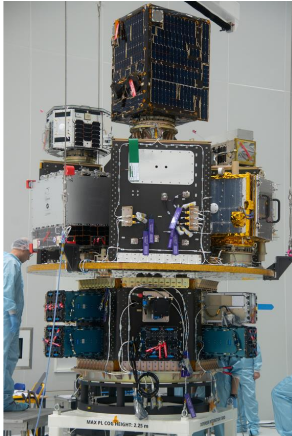
Fig. 6: Integration of satellites on Vega Dispenser in Europe's Spaceport in Kourou, French Guiana [15]
