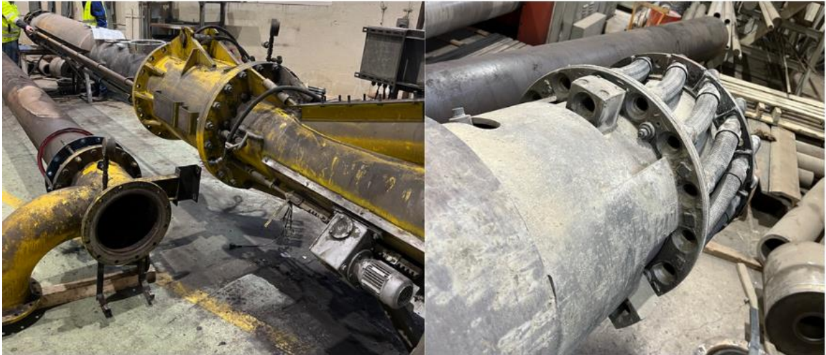
Fig. 17 Dismounted burner (“flexible hoses design”)
