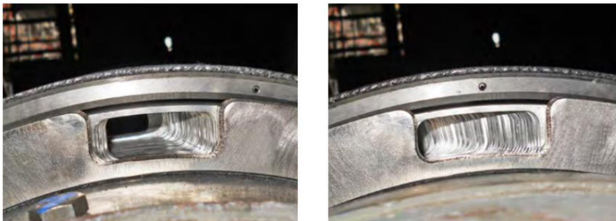
Fig. 15 Position „0“ (low swirl - long flame) vs Position „10“ (high swirl - short flame) [13]
