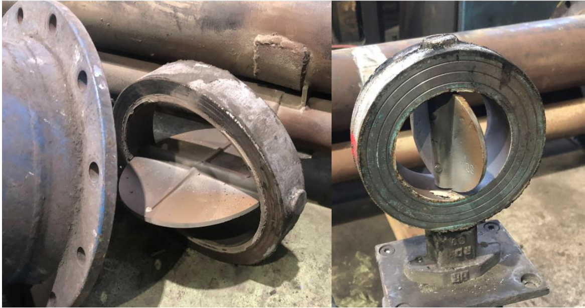
Fig. 29 Butterfly valves used in the burner channels
