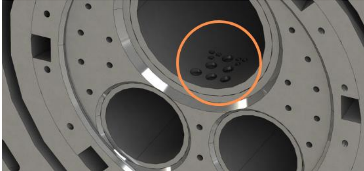
Fig. 22 Closer look at the RDF lifting pipe holes
