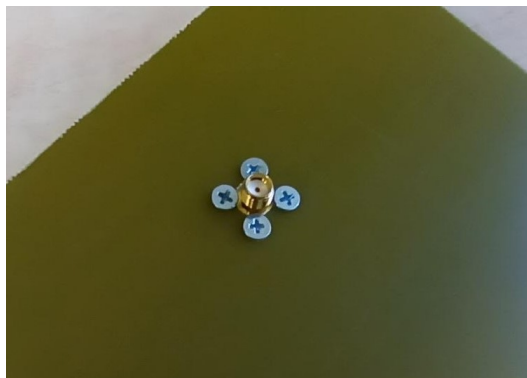
Fig. 6.9: Connectors are attached to the adapter with M3 Philips countersunk head screws
