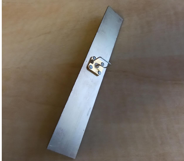
Fig. 6.8: Current loop fixed on the back side of the adapter
