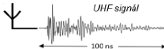
Fig. 2.11: Antenna measurement of complex response of partial discharge in time domain composed of directed and reflected waves inside transformer tank
