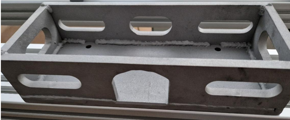
Fig. 42 Sand-blasted impact box.
