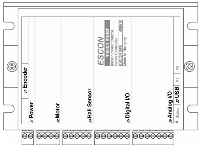
Figure 2.16: Motor driver ESCON 50/5 [20]
